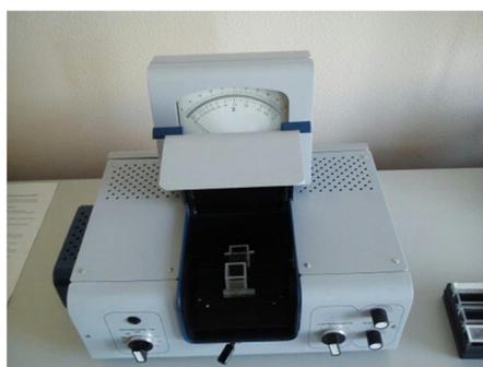
**Fig. 4.** Concentration photo-electric colorimeter CPC-2
