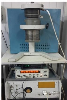
Fig. 1. Viscosimeter of constant strain VCS-0.2M
