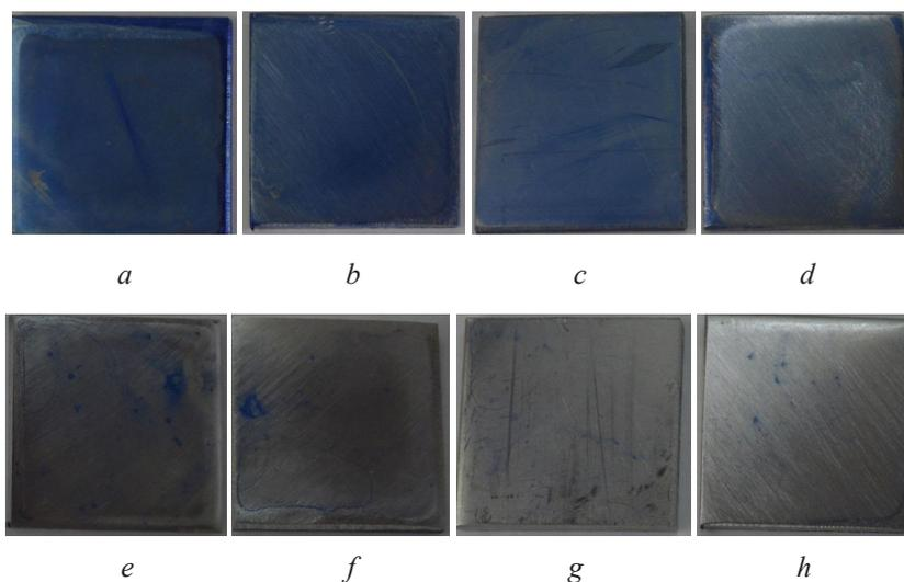
**Fig. 4.** Outlook of the stainless steel plates of different roughness, on which the biofilms of *S. Aureus* are formed *a, b, c, d* – before processing by *Savinase®Evity 16L* enzyme; *e, f, g, h* – after processing by the enzyme
