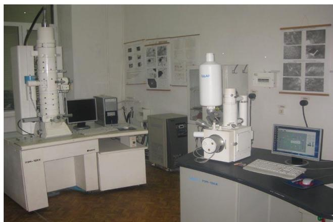
**Fig. 2.** Electric raster microscope (REM 106 I)
