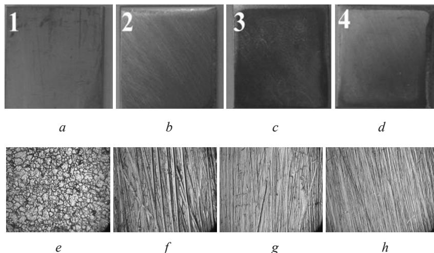
**Fig. 1.** Outlook of the plates of stainless steel AISI 321 with different roughness: *a, b, c, d* – native outlook of the plates; *e, f, g, h* – outlook of the plates under the microscope (magnification 1500 times)
