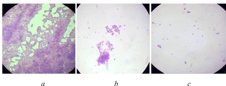
**Fig. 5.** Microscopic image of the biofilm conditions on the plates with different surface roughness: *a* – before processing by *Savinase®Eivity 16L* enzyme, *b* – after processing by the enzyme with surface roughness 0,63±0,87 mcm; *c* – at roughness 0,16±0,018 mcm (magnification 1350 times)
