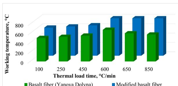
Fig. 9. Dependence of the working temperature of basalt fiber on the time of thermal load (T<sub>t,l</sub> – 1060 °C, Ø 180–250 microns)
