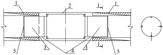
**Fig. 2.** Improved connection of circular hollow-core slabs with a monolithic girder in a precast-cast-in-place floor: 1 – slab supporting sections; 2 – monolithic girder; 3 – keys; 4 – cylindrical reinforcement cages; 5 – key size limiter
