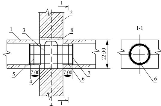
**Fig. 4.** Contact-platform joint of panel walls with hollow-plate support zones brought beyond the wall area: 1 – hollow-core slab; 2 – wall panel; 3 – stub bars from the wall panel; 4 – grouting concrete; 5 – key; 6 – key reinforcement cage; 7 – key size limiter; 8 – cement-sand mortar
