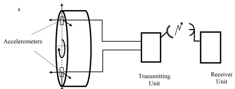
**Fig. 1.** Block diagram of the measuring unit
