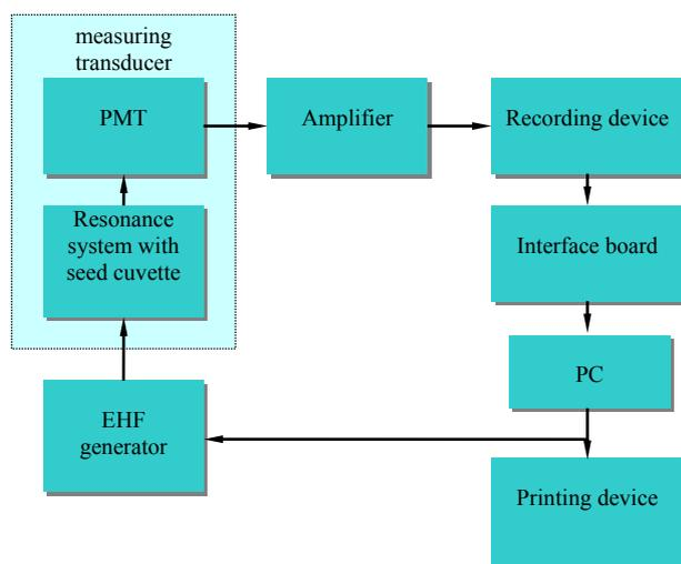
**Fig. 3.** Functional diagram of changes in the chemiluminescence of seeds
