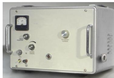
**Fig. 4.** General view of the device for measuring the chemiluminescence of seeds
