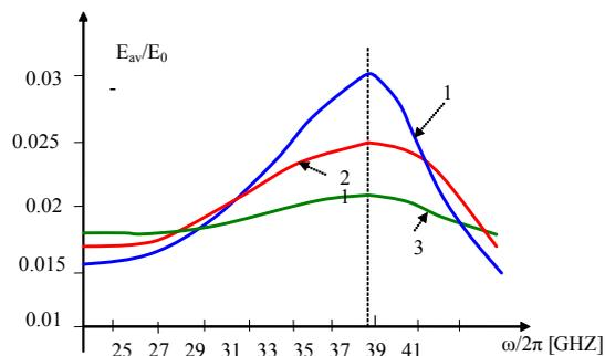
**Fig. 2.** Dependence of the normalized electric field averaged over the seed volume on the frequency of the exciting electromagnetic wave with the modulation frequency: 1 –  $\Omega=100$  Hz; 2 –  $\Omega=50$  Hz; 3 –  $\Omega=20$  Hz
